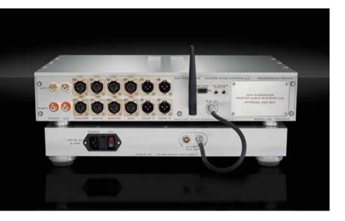
Like its bigger brother, the Progression power supply makes extensive use of electrical and magnetic shielding to keep radiated interference away from critical preamplifier circuits. Internal circuitry filters RF noise on the mains input, and compensates for asymmetric power waveforms and DC on the mains. A second DC output is included to power future Progression source components. It doesn't take a black belt in rocket surgery to get to the words 'phono stage' here.
